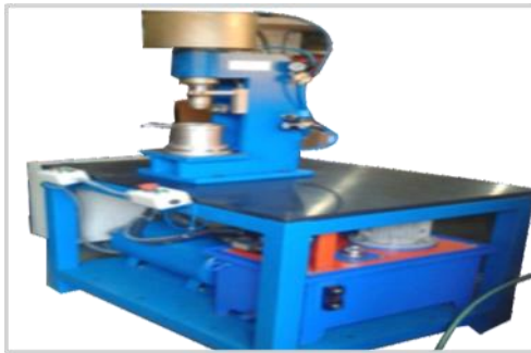
CAULKING EQUIPMENT Machine tool prototype factory, Ambernath
