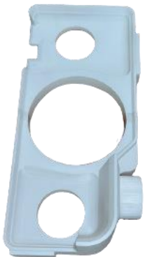
DEVELOPMENT OF GABLE (INVESTMENT CASTING) BY 3D PRINTING Gun Carriage Factory, Jabalpur
