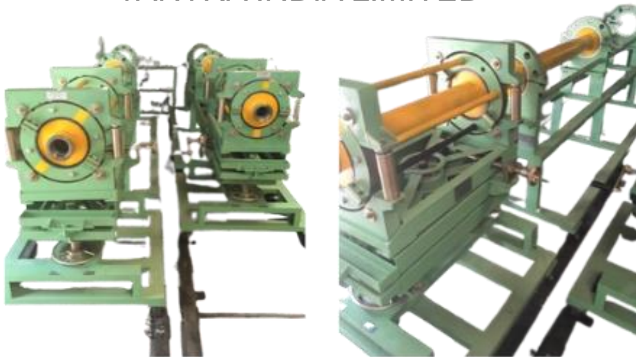
INTEGRATION TROLLEY FOR ASSEMBLY OF PINAKA WARHEAD & PROPULSION UNIT & DISMANTLING OF PINAKA ROCKET Ordnance factory Ambajhari, Nagpur
